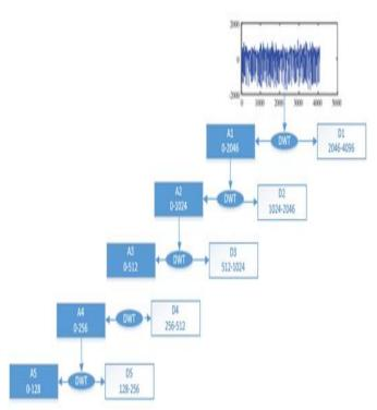
Figure 1: DWT Process [4].
